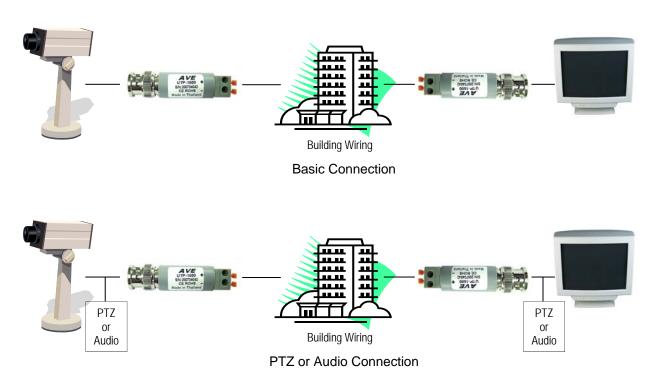
The AVE UTP-1500 module can be used as either a transmitter or receiver but is polarity sensitive. However reversing the wiring causes no ill effects to the device so if the picture is distorted just reverse the wires.
